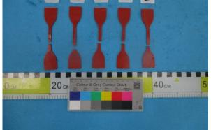
Before Test-Sample A- After Heat Ageing
