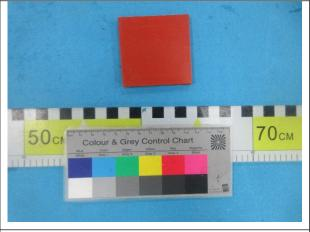
After Test-Sample A- After Heat Ageing
